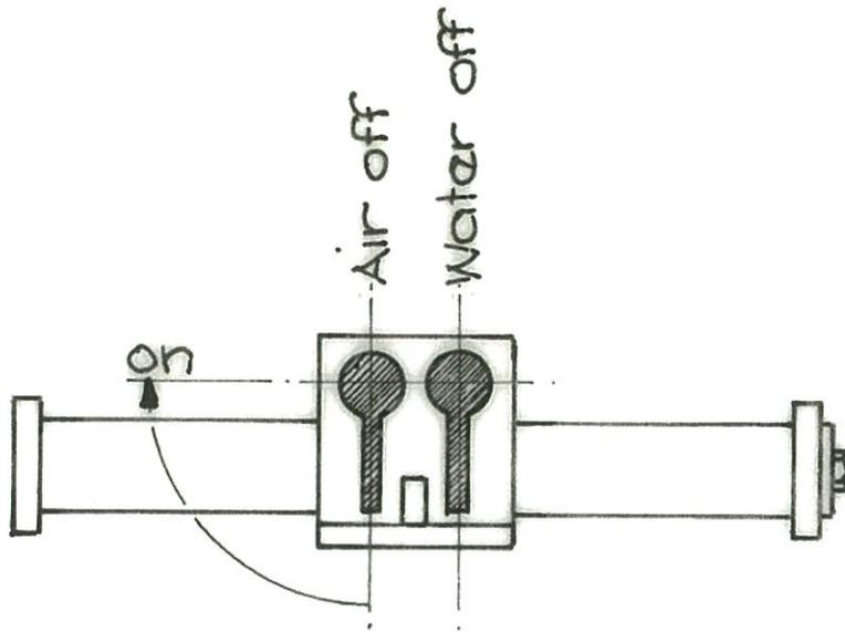
Figure 1: T-Bar control showing air and water ON/OFF positions
