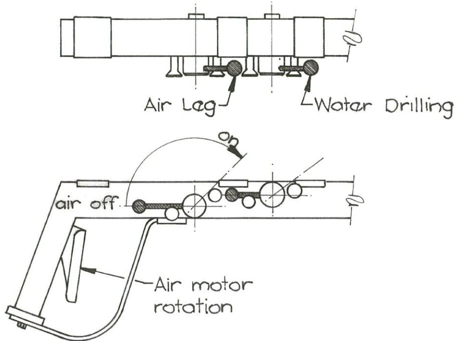
**Figure 4: Pistol grip arm in right hand configuration**
