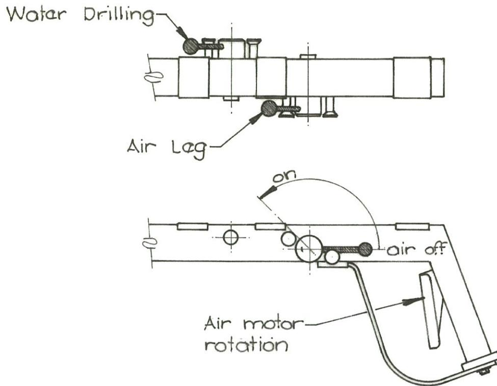
**Figure 3: Pistol grip arm in left hand configuration**
