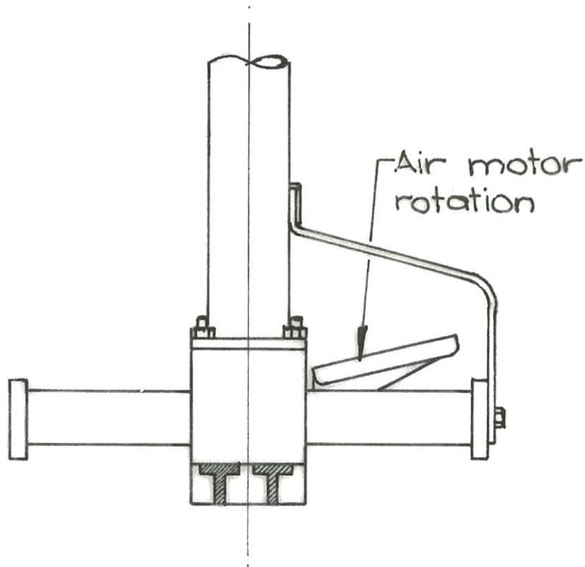
Figure 2: T-Bar control showing air motor rotation trigger
